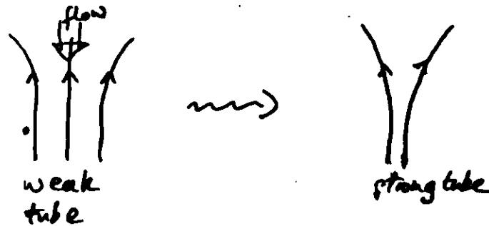
The 'collapse' of a weak tube to form a strong tube is a consequent of the convective instability in the tube
