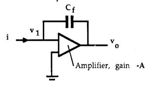
It has a very high input impedance without the feedback loop connected and therefore draws almost no current. The circuit equations are
