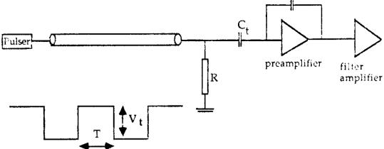
The input signal, usually a train of equal positive and negative going steps, is sent from a pulser via a cable terminated in its characteristic impedance, R. Even if the cable is too short to be considered as a transmission line it can be detached and terminated in the same resistance at a scope (i.e.  $50\Omega$  here) for proper observation of the signal.
