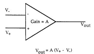
In reality the op-amp is never used in this simple way but is almost always used in a feedback mode where some fraction of the output voltage is fed back to the inverting  $(v_{-})$  input where it is subtracted from the input signal at this point. This is called negative feedback and explains why the inputs are labelled as + and -: the output goes positive when the non-inverting input  $(v_{+})$  goes more positive than the inverting input  $(v_{-})$ , and vice-versa.
