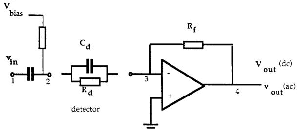
The circuit forms an amplifier with a gain  $G = -R_f/Z_d$  where  $Z_d$  is the impedance of  $C_d$  and  $R_d$  in parallel (Appendix B).
