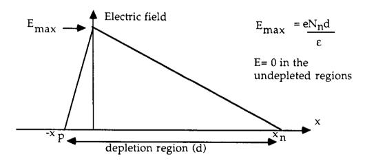
The potential difference across the junction can be obtained by inspection (the area under the triangle) to be:
