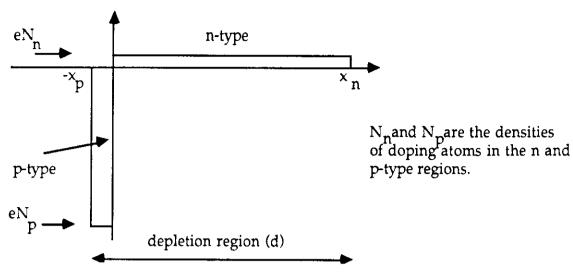
Overall charge neutrality requires  $N_p x_p = N_n x_n$ . The electric field and potential are calculated from Poisson's equation
