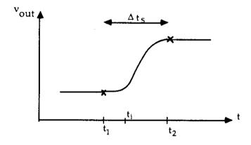
The output from a charge sensitive preamplifier is given by  $v_{out}$  and the expected arrival time of an interaction time is accurately known to be  $t_i$ .
