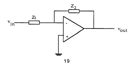
$$v_{-} = v_{+} = 0$$
