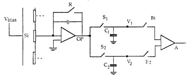
In addition to the normal charge-sensitive preamplifier there are a number of important switches. These are actually FETs (Field Effect Transistors) which can be switched from a conducting to a non-conducting state by application of a voltage to the gate.
