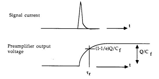
In practice the feedback loop of the preamplifier usually also includes a large resistor in parallel with the capacitor so that the preamplifier output pulse actually decays exponentially from its peak value with a long time constant.
