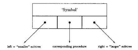
The upper box (8 characters?) contains the characters of the symbol. The next three boxes contain pointers, that is addresses of other boxes (left and right subtree), or of the code (procedure) associated with the symbol.
