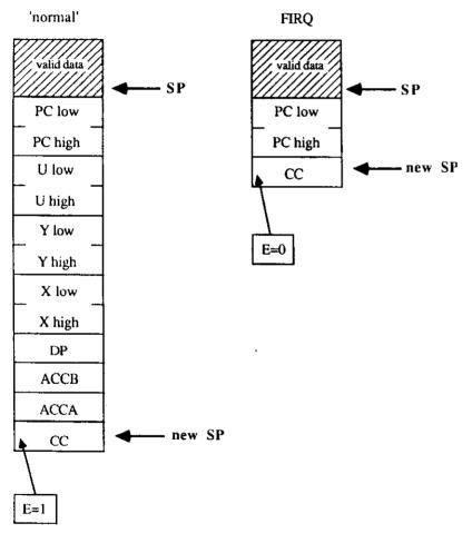
When 'RTI' is executed, CC is pulled first and therefore the CPU will know, if all registers have to be recovered or only the PC in the case of the FIRQ.
