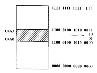
A 15 A 14 A 13 A 12 A 11 A 10 A 9 A 8 A 7 A 6 A 5 A 4 A 3 A 2 A 1 A 1 A 10 Base Address Internal Address
