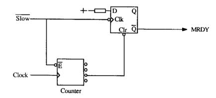
The SLOW signal is generated by the decoder detecting that the CPU wants to address the slow device. The delay needed can be adjusted using different outputs of the counter.
