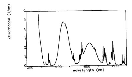
Fig. 7. Absorption of Nd, Cr: GSGG
