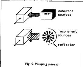
The incoherent sources are by far the most used up to now, because of their lower cost and easier availability. The maximum average power available from lamp pumped solid state lasers is also order of magnitude higher than that available from laser pumped systems. This situation is now evolving, because of the recent availability of relatively high power semiconductor lasers. but their high cost limit the average power level in the watt range, at least up to now.
