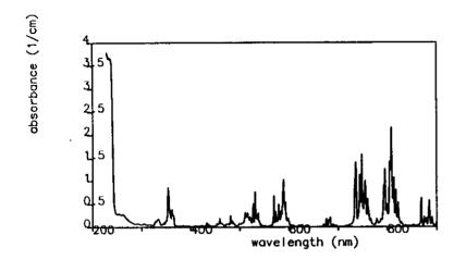
Fig. 5. Absorption of Nd:YAG
