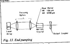
In its most basic form, end pumping involves (fig. 13) a collimating lens with a large numerical aperture in order to collect radiation from a large cone angle, and a focusing lens to produce a small diameter spot inside the laser crystal. Since the radiation lobe emitted from a diode array has a high degree of astigmatism, one can introduce prisms or cylindrical optics to
