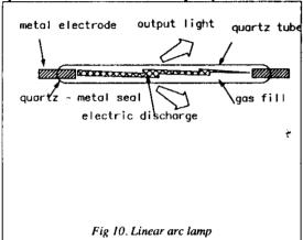
A linear or flash lamp is basically very simple. A quartz tube is ended by two metal electrodes and filled with a rare gas (krypton or xenon) at a pressure from 4 bar (for CW arc lamps) to about 0.5 bar (for short pulse arc lamps.
