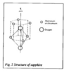
the so-called c axis, which forms the major diagonal of the unit cell. Since the crystal is uniaxial, it has two indices of refraction, the ordinary ray having the E vector perpendicular to the c (optic) axis, and the extraordinary ray having the E vector parallel to the c axis.
