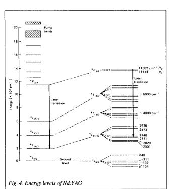
quality and has a high thermal conductivity. Furthermore, the cubic structure of YAG favors a narrow fluorescent line-width, which results in high gain and low threshold for laser operation. In Nd:YAG, trivalent neodymium substitutes for trivalent yttrium, so charge compensation is not required.
