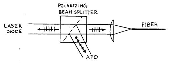
THE 4% REFLECTION POWER HAS THE SAME POLARIZATION THAN THE L.D. POWER, INSTEAD THE SCATTERED POWER IS NOT POLARIZED.
