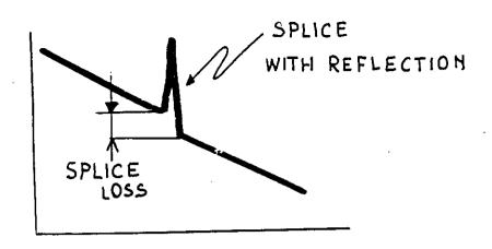
SPLICES ESTWEEN INFFERENT FIBERS BUT WITH EQUAL REFRACTIVE INDEX (ML) AND DIFFERENT MODE SPOT RADIUS (W).
