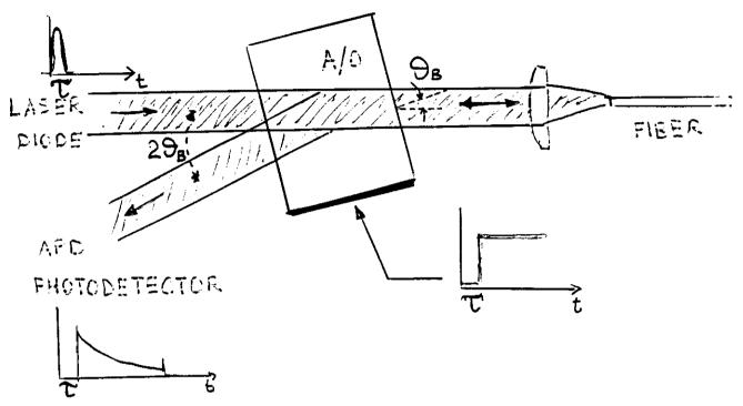
OST STHE OPTICAL PULSE OF THE LASER TRAVELS THE A/O MODULE LATOR, AHD ARRIVES ON THE FIETH.
