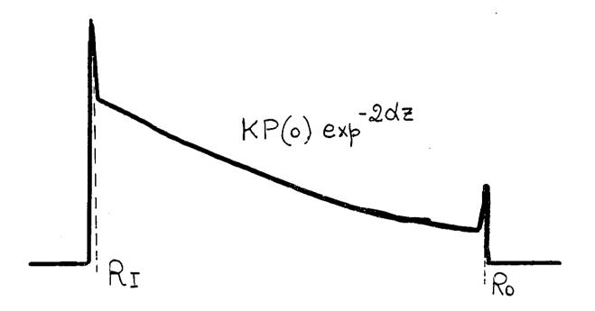
RI AND RO ARE THE REFLECTIONS AT THE INPUT AND THE OUTPUT FIBER END.
