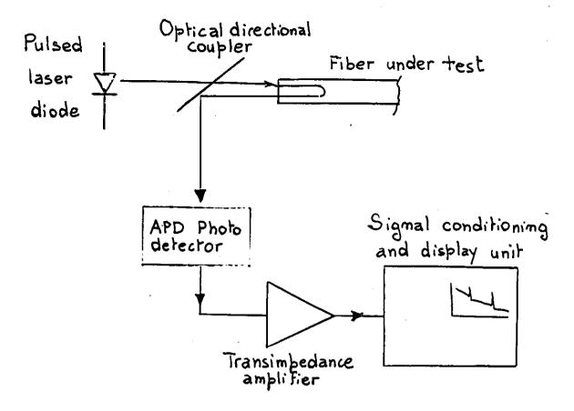
Source: - pulsed laser diode - peak power 1:10mw - bulse width depends on the measurable range (for high resolution instrument from 3 to 10ms, for long distance instrument 1 + 4 Ms).
