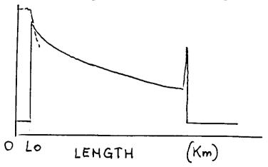
OPTICAL LINK MEASURED WITH AN O.T. D.R.
