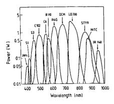
Pump power: 3 W in the UV, 4 W in the visible, 2 W in the infrared. Energy conversion efficiency: up to 40 %.
