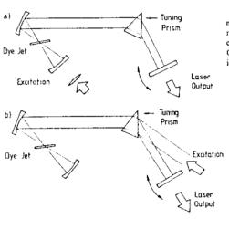
Tunable three-element dye laser resonator using reflecting optics. (a) Collinear excitation through end mirror. (b) Collinear excitation through tuning prism
