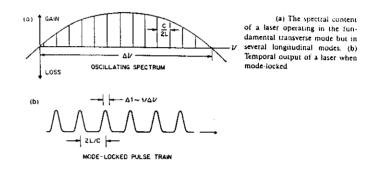
In case of a single pulse in the optical cavity, the period of the pulse train is T = 2L/c. The width of the pulses is inversely proportional to the width of the oscillating spectrum. Because this extends with dyes over nearly 100 nm, the optical pulses can be as short as 10 fs.
