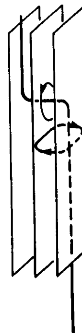
Fig.9: Kink motion of a vortex with core parallel to the planes.
