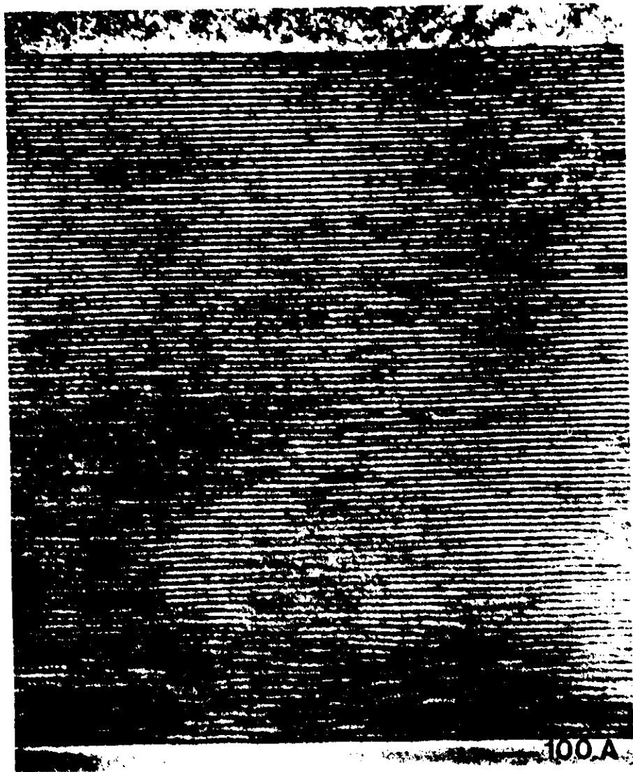
Figure 19: TEM micrograph of a GaAs(3 \mu m)/AlAs(3 \mu m) superlattice
