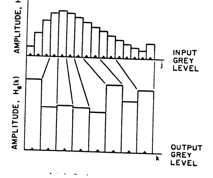
point transformation G(x,y) = h(f(x,y)), where f(x,y) is the input image, G(x,y) is the enhanced image and h is the transformation function.
