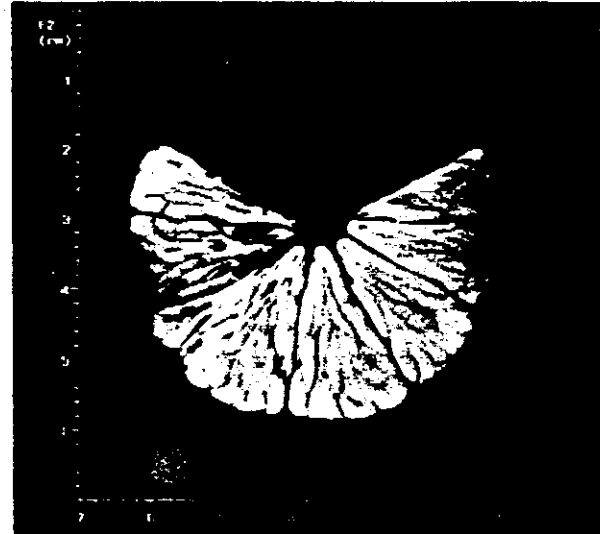
Figure 1 Proton NMR image (7.0 Tesla, 300 MHz) of a 2-mm slice of a navel orange that had a notch cut in it. Notice that the seeds, membrane structures, and features of the peel are visible in this presentation.
