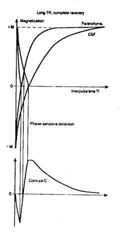
Find the time delay Ti. where the FID signal equals zero.
