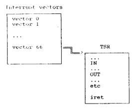
A particular case of hardware activated TSRs are those woken up by a "hot key". Each time a key is pressed or released it produces an INT 9. The TSR can sheak into the chain of events associated with vector 9 and have a look at the keystroke before any other program gets a chance to read (and thereby destroy) it.
