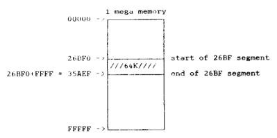
Within this 64K segment IP defines an offset: IP = 0000 addresses the first location (26BF0) . IP = 0001 the next (26BF1) and so on until the last which corresponds to IP = FFFF .
