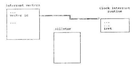
What our program could have done before exiting with the 31H function is to set up the vectors like this:
