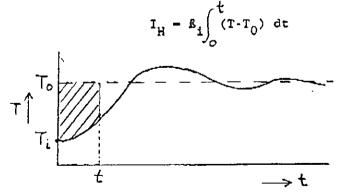
The system's temperature will now evolve in time as sketched in the figure. At a time t the heater current is proportional to the shaded area. Conse-
