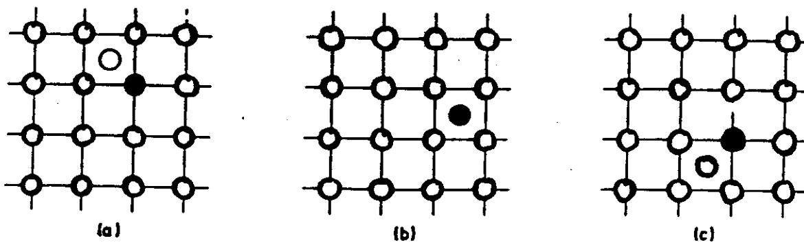
indirect interstitial mechanism (= interstitialcy mechanism)
