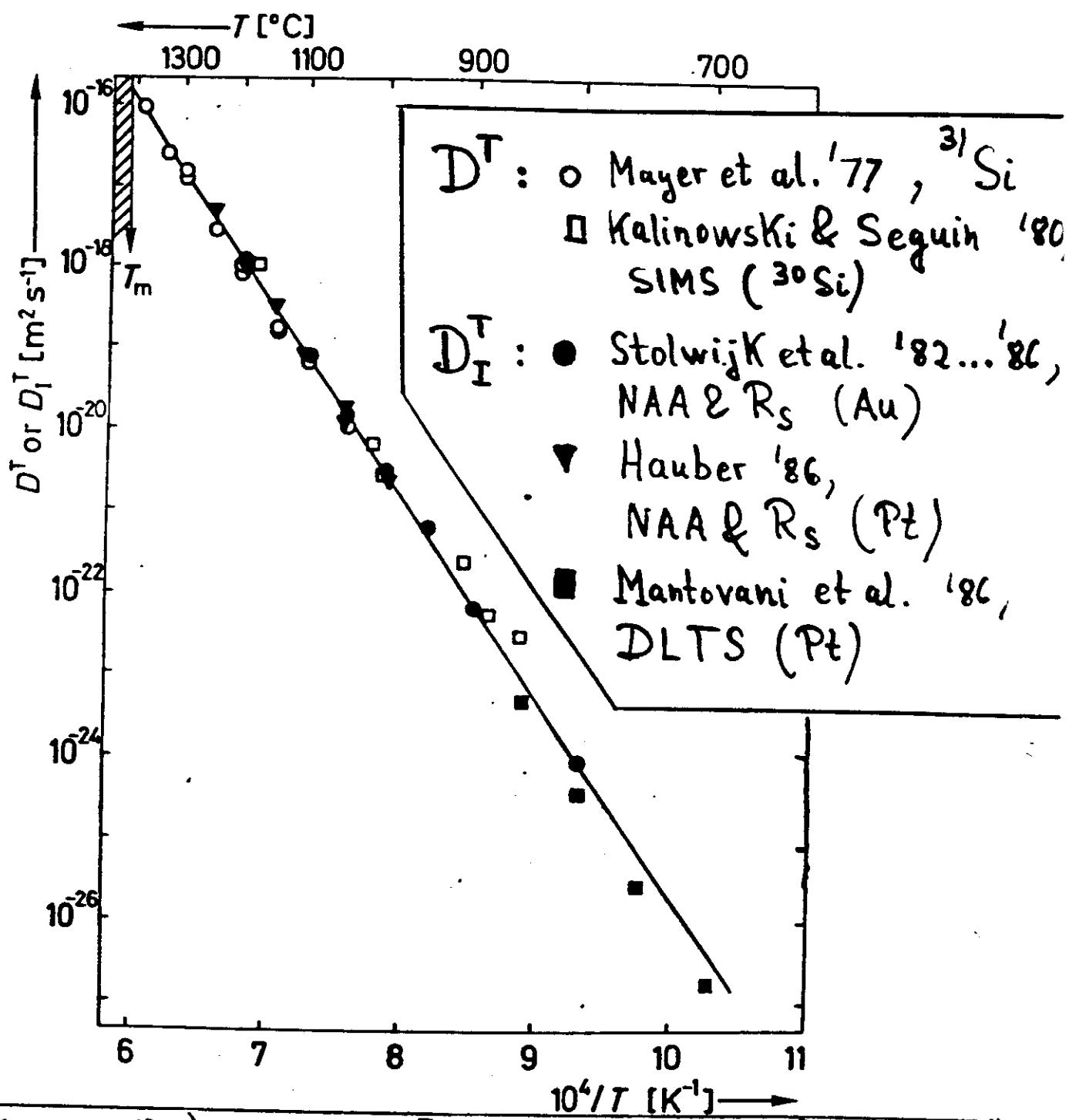
$$D^T = (14.6 \pm 1.7) \times 10^{-2} \exp \left[ -(5.02 \pm 0.10) \text{eV}/kT \right] \text{m}^2/\text{s}$$
