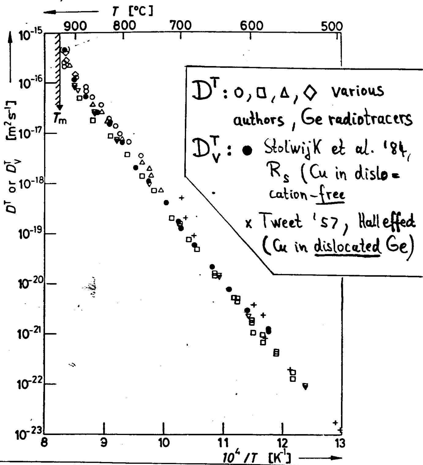
$$D^T = (1.36 \pm 0.15) \times 10^{-3} \exp[-(3.09 \pm 0.02) \text{eV}/kT] \text{ m}^2/\text{s}$$
