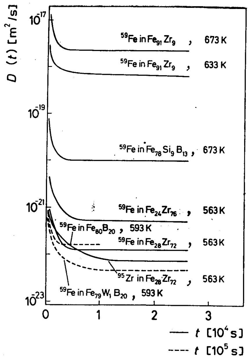
Schematic illustration and description of the isothermal change of the diffusivities in amorphous alloys
