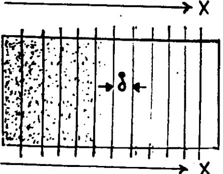
sectioning and measurement of radioactivity of the individual sections
