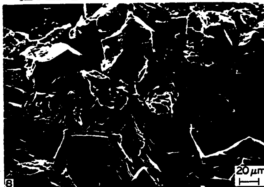
FIG. 7. Fracture surface of a Type AISI 304 stainless steel wire stressed in fresh 40% \text{MgCl}_2 solution at 100°C. Potential, -0.175 \text{ V(NHE)} ; strain rate, 1.5 \times 10^{-5} \text{ s}^{-1} ; failure time, 94 min.
