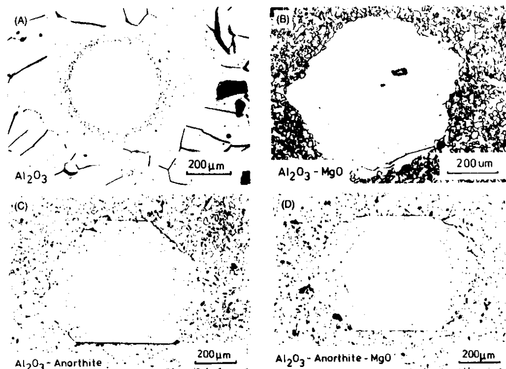
Fig. 3. Alumina with single-crystal seeds after hot-pressing (35 MPa) at 1800°C: (A) \text{Al}_2\text{O}_3 , 60 min; (B) \text{Al}_2\text{O}_3 + 0.1 wt% MgO, 60 min; (C) \text{Al}_2\text{O}_3 + 1.0 wt% anorthite, 10 min; (D) \text{Al}_2\text{O}_3 + 0.9 wt% anorthite + 0.1 wt% MgO, 10 min.
