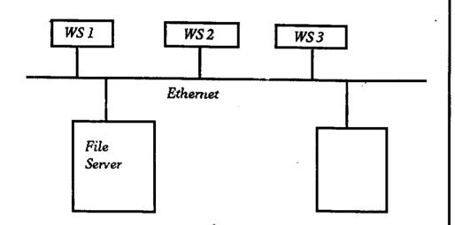
On startup the workstation sends a boot request down the ethernet containing the requesting node's hardware address. It's server recognizes the request and downline loads the kernel image corresponding to the workstation's hardware configuration.
