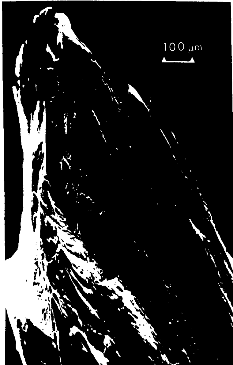
FIG. 5. A chisel point formed in a rod specimen of gold after necking and rupture. Original specimen was 0.15 cm in diameter (courtesy of H. Wilsdorf 6 ).
