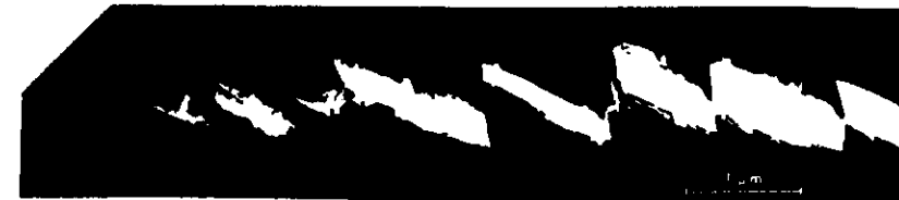
FIG. 14. Side view of a growing fracture in a thin film of gold. Holes are shown nucleating ahead of the crack (see Lyles and Wilsdorf 12 ). (Courtesy of H. G. F. Wilsdorf.)
