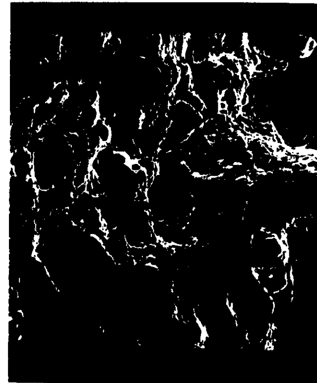
FIG. 6. Ductile fracture surface, showing the final dimpled structure of hole growth. Precipitate particles are visible in some of the dimples which served as nucleation sites for the holes (courtesy of C. Interrante).
