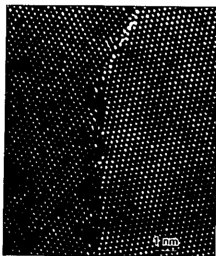
Figure 4. HREM micrograph of (1\bar{1}0) tilt GB in Au, showing a short symmetric (221) facet near the top of the figure and an asymmetric (557)(771) facet with the same misorientation [ \Psi \approx 39^\circ ( \Sigma 9 )]. White spots represent atomic columns.
