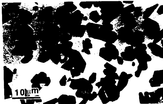
Figure 2. Cavity formation in Carborundum KX01. This material contains \approx 33 vol. % silicon. Cavities are always located at Si/SiC interfaces, most often between two closely spaced SiC grains. As the cavities grow from the narrow space between the grains, they arrest on encountering a larger pool of silicon. The applied tensile stress was vertical (top to bottom) in the figure.
