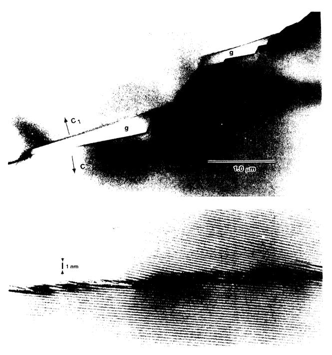
8. Partially-wetted boundaries between the two sapphire crystals. (a) glass pockets, g, are bounded by (0001) and  $(1\bar{2}13)$  planes. The glass pockets are connected by a low-angle grain boundary; (b) partially-wetted boundary with very little glass at the boundary.
