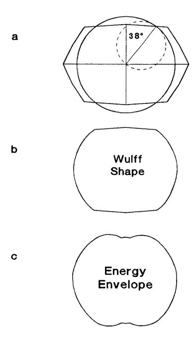
13. (a) Comparison of a low-angle grain boundary Wulff shape (large circle) with the Wulff shape of a wetted, facetted bicrystal boundary. The two figures are scaled so that the grain boundary Wulff shape intersects the bicrystal Wulff shape at 38°. The inner envelope of the two overlaid Wulff shapes, (b), is the Wulff shape of the interface. Between angles of 3.5° and 38°, the lowest energy is obtained for a partially-wetted interface. The energy of the interface is shown in (c).
