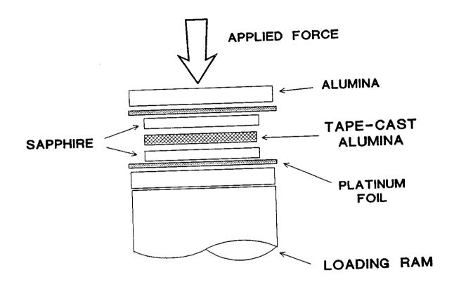
1. Experimental configuration to produce sapphire bicrystals with anorthite glass at the interface.
