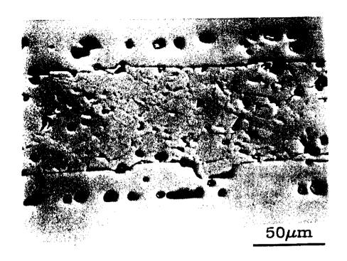
2. Microstructure of sapphire specimens with vitreous grain boundaries; 2h of sintering at 1650°C with 7 MPa compressive stress applied normal to the interface.
