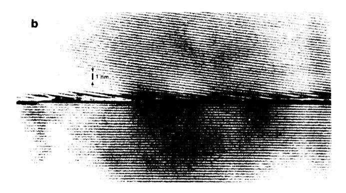
6. Fully-wetted boundaries between the two sapphire crystals. (a) extremes of structure; (b) boundary with very little glass at the interface.
