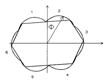
11. Wetted bicrystal boundary energy is determined from the two surface energy curves, tilted relative to each other. The energy of the wetted boundary is obtained by adding the energies of the two solid-liquid interfaces as a function of the angle,  $\Phi$ .
