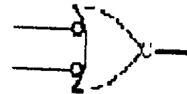
Fig. 3.6. Realizations of logical OR for eight choices of voltage.
