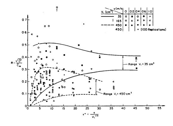
Figure 5-14. Concentration variance ratio,  $\sigma_{\rm C}/{\rm C}$ , versus downwind distance, observed by Meroney and Lohmeyer (1984) in a wind tunnel. The source is an instantanteous dense gas cloud.
