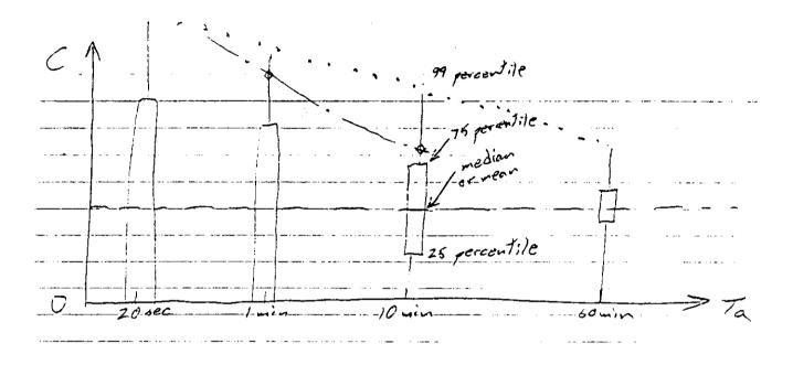
Figure 2. Typical distributions of concentration observed at a given monitor location, for various averaging times, T<sub>a</sub>. The dashed line goes through the means at each T<sub>a</sub>, and the dotted line goes through the 99th percentile of each distribution. The dashed-dotted line goes through the maximum at that T<sub>a</sub> assuming the sampling time is 60 min.
