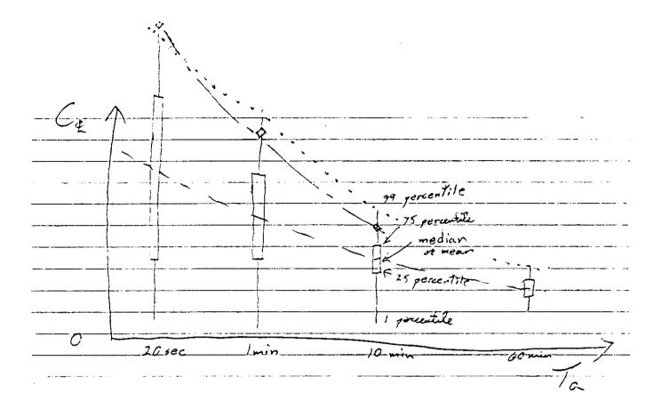
Figure 1. Typical distributions of centerline concentration,  $C_{co}$  at a given x, for various averaging times,  $T_a$ . The dashed line goes through the means at each  $T_a$ , and the dotted line goes through the 99th percentile of each distribution. The dashed-dotted line goes through the maximum at that  $T_a$  assuming the sampling time is 60 min.
