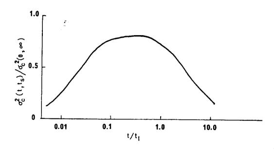
Figure 5-15. Fraction of total possible concentration fluctuation variance from Eqs (5-60) and (5-61), as a function of sampling time  $T_{\rm S}$ , averaging time T and integral time scale  $T_{\rm I}$ . It is assumed that  $T_{\rm S}/T_{\rm I}$  = 100.
