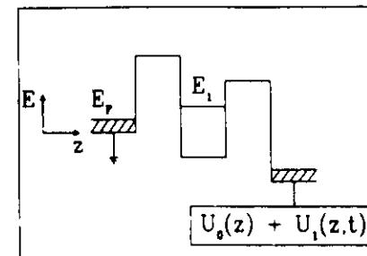
HF field modulates  $U$  with  $H_1 = U_1 \cos \omega t$
