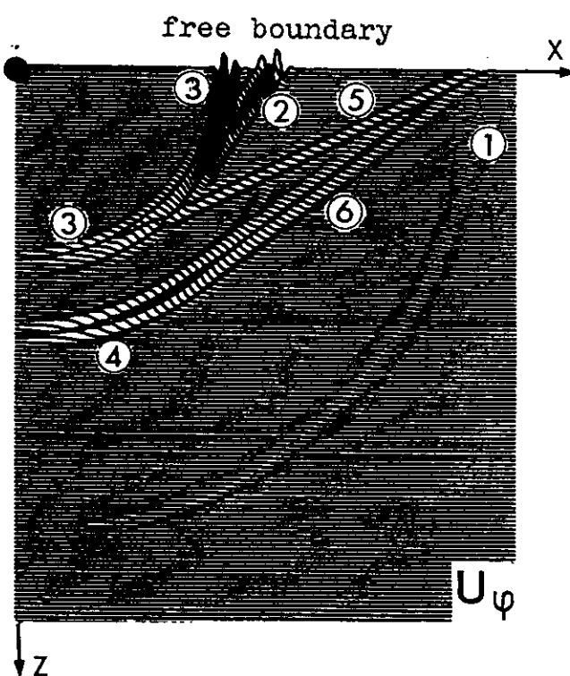
Fig. Snapshots of the vertical plane ( $\varphi = 80^\circ$ ) of three displacement components at the fixed moment of time for the anisotropic model of the medium.
