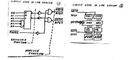
READ IN THE VALUE OF A SET OF SWITCHES AND OUTPUT THAT VALUE THE 'LED' DISPLAY.
