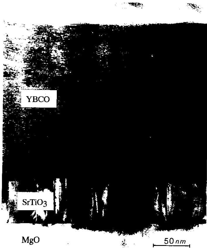
Figure 14. TEM picture of the YBCO/SrTiO 3 /MgO cross-sectioned sample of Figure 8. (Courtesy of A. Migliori)
