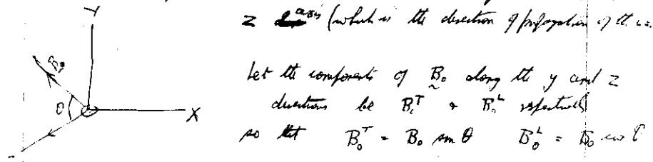
Let the components of  $\underline{B}_0$  along the y and z directions be  $B_0^T$  &  $B_0^L$  respectively
