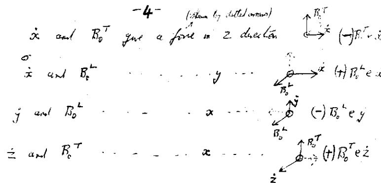
i.e. the external magnetic field in the plane OYZ (i.e. with components in the Y & Z directions only) gives rise to one force term in the y + z direction and the force term in the x direction.
