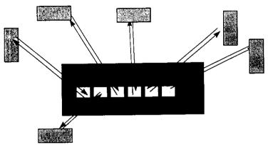
The hub retransmits on all his ports (except input one) every input Collisions as usual detected only by hosts, never by hub Hub extends jam, like repeaters
