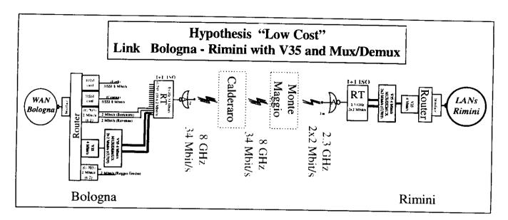
Considering this architecture, we can consider a V35 interface on the router in Rimini for a 4 Mbit/s flow, which enters in a multiplexer dividing the flow into two HDB3 2 Mbit/s flows. These two flows enter separately into the transmitter, through which they are sent to Bologna. Here another multiplexer unify the two flows in the original one which finally enters in the V35 interface of the router.
