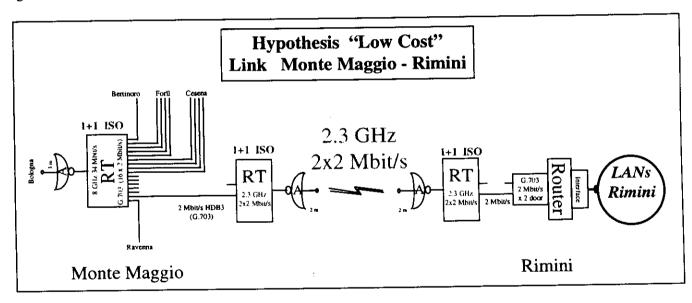
We can notice that the band expected for this link, would permit to transport two 2 Mbit/s flows, but the second isn't used because the router in Rimini isn't able to manage two different interfaces. In order to exploit both the interfaces for the flows in the two directions (from Rimini to Bologna and from Bologna to Rimini) we would add two multiplexer/demultiplexer (one in Bologna and one in Rimini) and two V35 interfaces (one on the router in Bologna and one on the router in Rimini).
