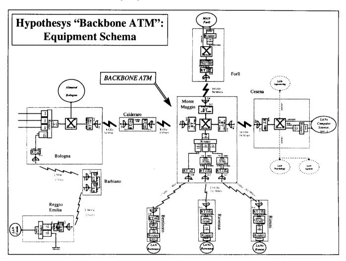
In particular, it must be pointed at the Backbone in ATM technology between Bologna and Monte Maggio. It devides and follows towards Cesena and Forlì, constituting a high-speed backbone between Bologna and Monte Maggio.
