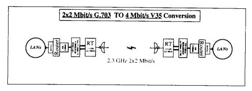
The connection between a 34368 Kbit/s RTX and a router is possible instead, because the routers have got interfaces which accept this kind of size; in particular the ATM standard contemplate 34368 Kbit/s HDB3interfaces for connecting to the routers.
