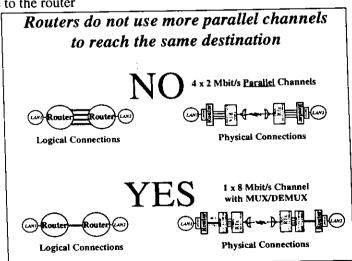
In a similar manner, the connection between a 2x2048 Kbit/s HDB3 RTX and a router is difficult to execute; indeed it is not possible to enter directly into the router with two flows of 2048 Kbit/s each one, because the router
