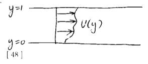
For simplicity, we will consider the idealized case of flows confined between two rigid vertical walls at y = 0 and y = 1 (channel flow), where we apply the boundary conditions
