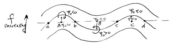
The velocity field at A' will cause a to go up, b to go down, and the velocity field at B' will cause b to go down, c to go up, so that the entire wave will go towards the left (west). We can also think of the flow pattern as a vortex street which self-advects to the west.
