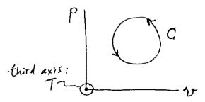
Note the state equation f(p, v, T) = 0 defines a surface in p, v, T coordinates for fluids of fixed composition. Then,
