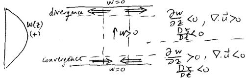
In the case of descending motion we must have the opposite case for upper lower parts, so that vorticity increases in the upper part, and decreases in the lower part:
