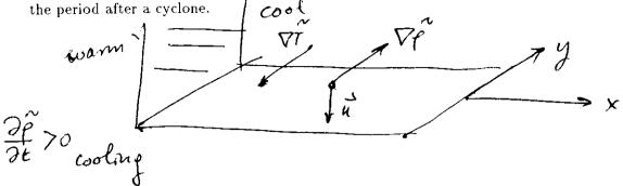
One of the most basic relationships is that of thermal wind, simply combining the geostrophic and hydrostatic relations:
