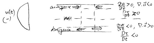
Therefore, if the fluid is bounded between two horizontal surfaces, we expect *phase shifts* between motions near top and bottom parts of the fluid motion. This *slanting* of motion results from different rates of the change of vorticity at different vertical levels. While the vorticity of a wave motion may be decreasing near the bottom it would tends to increase near the top, and *vica versa*.
