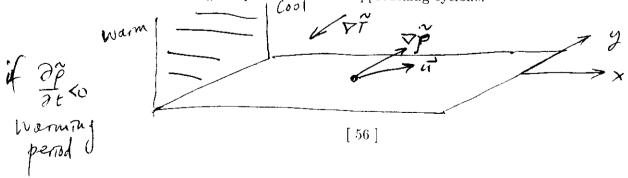
On the other hand if there is a cooling situation  $(\partial \tilde{\rho}/\partial t > 0)$ , we must have  $\vec{u} \cdot \nabla \tilde{\rho} < 0$ , i.e., the vectors  $\vec{u}$  and  $\nabla \tilde{\rho}$  must have components pointing in the opposite direction. This means that the flow must have a component from north to south, i.e. we must have cold advection, such as during the period after a cyclone.
