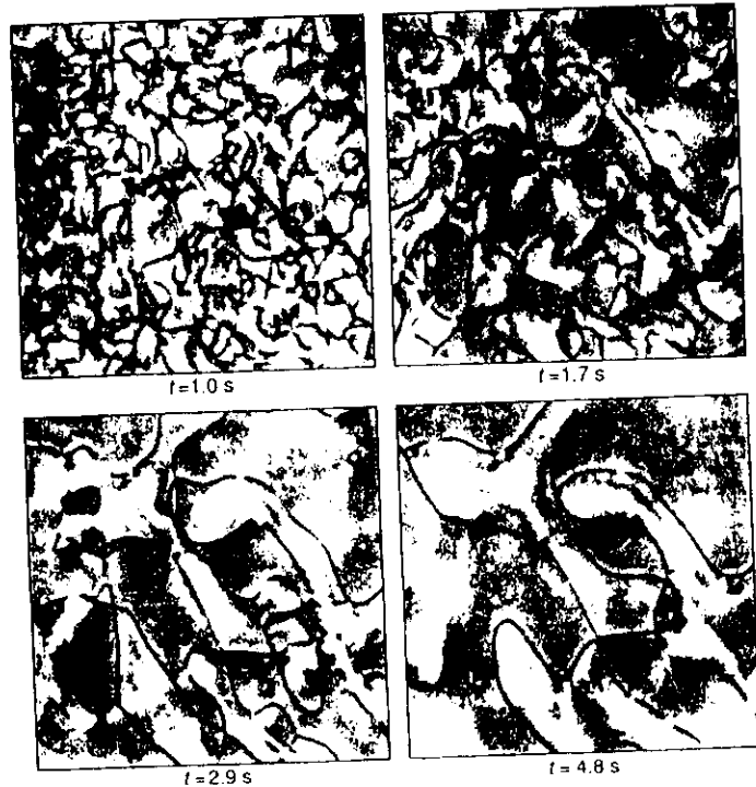
Fig. 4. A coarsening sequence showing the strings visible in our 230- \mu\text{m} -thick pressure cell containing K15 nematic liquid crystal, at t = 1.0, 1.7, 2.9 , and 4.8 seconds after a pressure jump of \Delta P = 4.7 MPa from an initially isotropic state in equilibrium at approximately 33^\circ\text{C} and 3.6 MPa. The evolution of the string network shows self-similar or "scaling" behavior. Each picture shows a region 360 \mu\text{m} in width.
