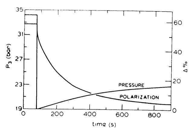
A rapid-melting experiment to produce highly polarized quid  ${}^{3}\text{He}$ :  $P_{3}$  and  $\Delta$  vs. time.
