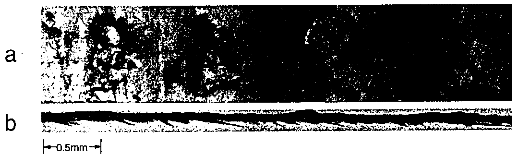
FIG. 15. (a) A top (XZ plane) view and (b) a side (XY plane) view of a section of the surface formed by a crack moving with velocity of 600 m/s in a 0.8-mm-thick plate. Note the appearance of large branches beneath the "cleavage zones" on the fracture surface. We view the large "upheavals," situated above the large microbranches on the fracture surface, as marking the onset of microbranches that penetrate the opposing crack surface.
