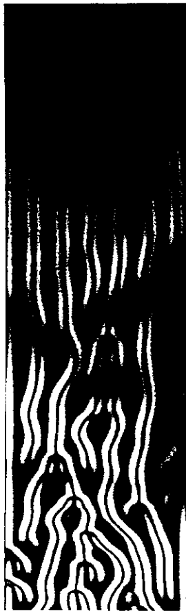
Fig. 6. Time evolution of the phase turbulence under increasing control intensity. The square of the flux j is shown in gray scale; the parameter \mu is increased with speed \epsilon = 3 \times 10^{-4} from zero (the left side) to \mu = 0.03 (the right side), other parameters are \beta = -0.8 , r = 2.0 and \chi = 0 .
