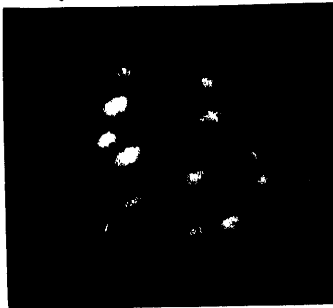
Figure 1(a) STM image of surface of 2.4 monolayers of InAs on GaAs (square size 1000 \text{ \AA} \times 1000 \text{ \AA} ).
