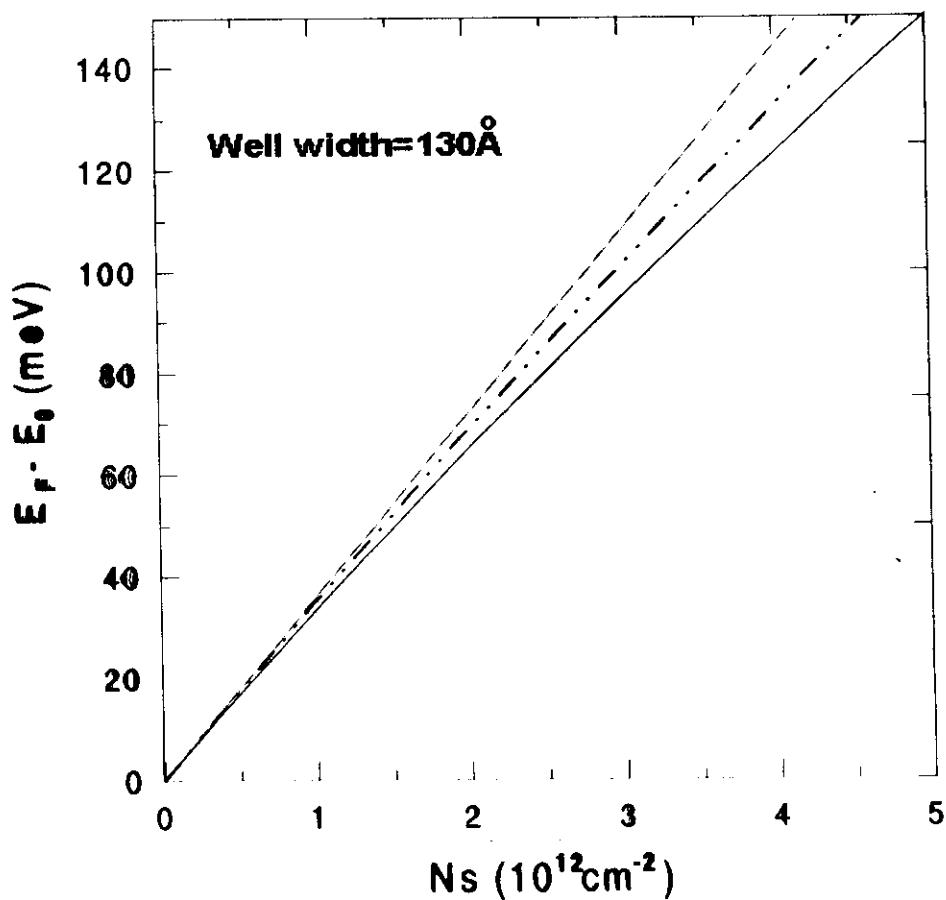
*variation of the Fermi level position from the first electronic subband*
