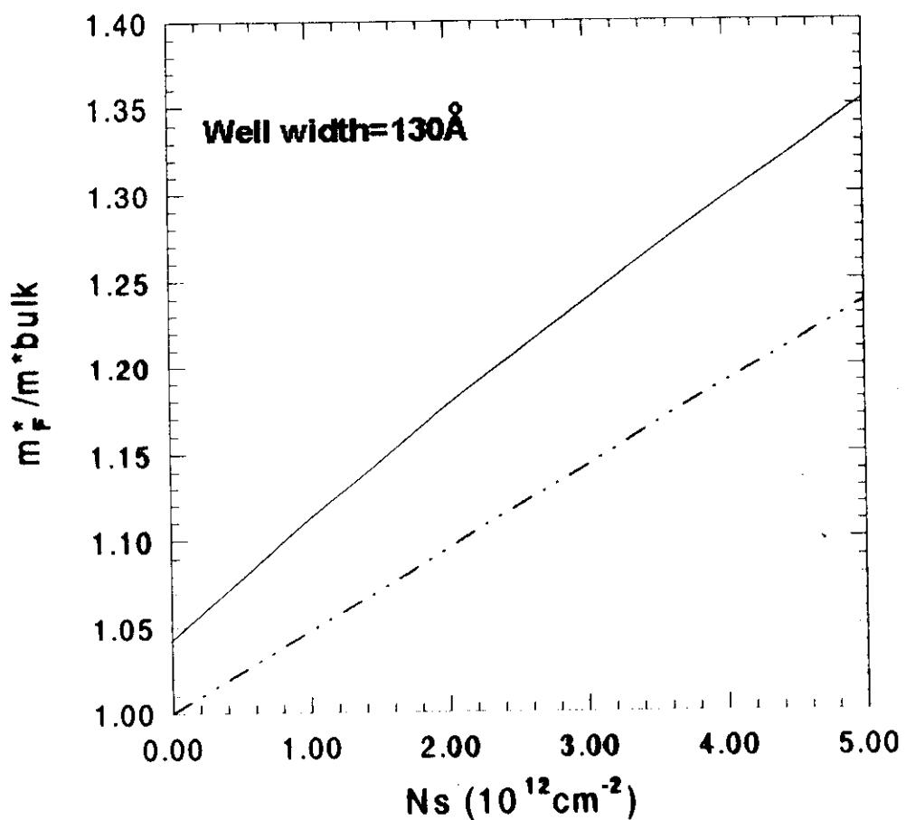
**variation of the Fermi level effective mass with first subband carrier density using modified Kane model (solid line) and Kane model with experimental values of Eg and m\* (dashed line)**
