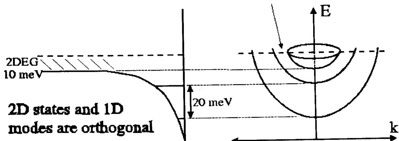
**Electrons confined to 1D modes even in the presence of the 2DEG**
