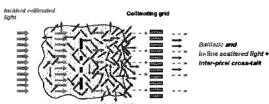
Suitable for weak scattering – applied to X-ray imaging
