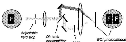
Multi-spectral imager provides 2-channel (up to 8) spectral resolution
