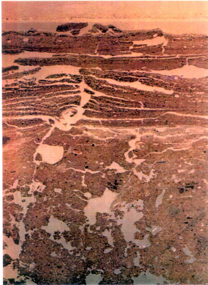
Figure 9 - Macrophotograph of a vertically oriented thin section from undisturbed surface samples of a cultivated loam soil. The presence of a very thick surface crust is very evident. However, the presence of organic material can cause vertical cracks in the compacted layers, thus creating the continuity in a vertical sense very important for water infiltration and seedling emergence. Picture taken under a macro-epidiascope with plain polarised light. Frame length 3 cm.
