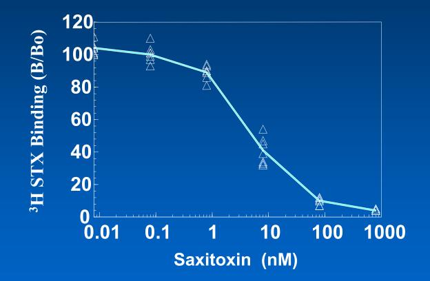
$K_i = 3.66 \pm 0.86$  nM in 7 independent assays run of different days Limit of detection ~5 ng/ml in a sample extract
