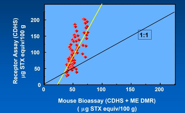
\*\* undiluted sample matrix may cause underestimate in mouse bioassay < 80 mg/100 g shellfish NOTE: Similar discrepancy observed HPLC vs mouse bioassay (Study currently pending availability of <sup>3</sup>H STX)
