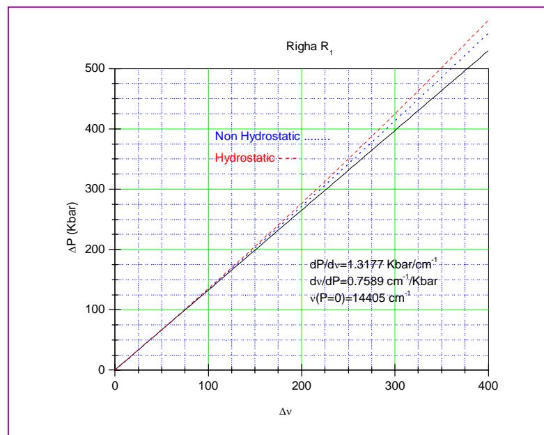
Pressure measurement by frequency shift
