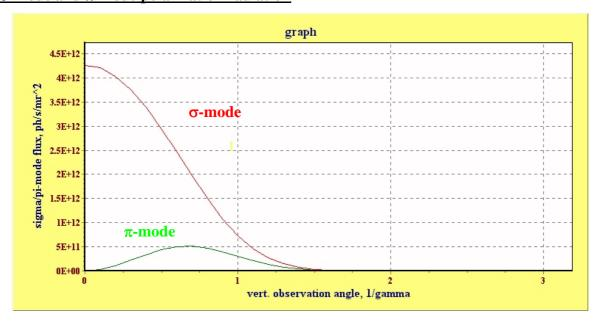
$\sigma$ -mode and  $\pi$ -mode radiation as a function of vertical observation angle(in unit of  $1/\gamma$ ) for the case of photon energy equals to the critical photon energy.
