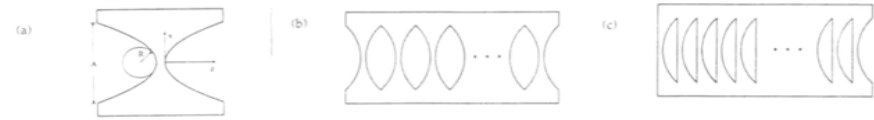
Fig. 3. Schematic view of the parabolically shaped single and compound refractive lenses: R , radius of curvature; A , aperture of the lens; p , length of the single lens or the distance between the centers of the two neighboring holes for a compound lens. (a) Single parabolic refractive lens, (b) compound refractive lens with parabolically shaped holes, (c) compound refractive lens with parabolically shaped half-holes.
