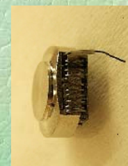
Nickel sample with the filament for DC resistive heating and pulsed current magnetizing remanence ~30%
