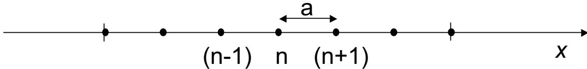
$$-\frac{\hbar^2}{2m^*} \frac{d^2\psi}{dx^2} + E_C \psi = E \psi \rightarrow -\frac{\hbar^2}{2m^*} \left[ \frac{\psi_{n+1} - 2\psi_n + \psi_{n-1}}{a^2} \right] = (E - E_C) \psi_n$$
