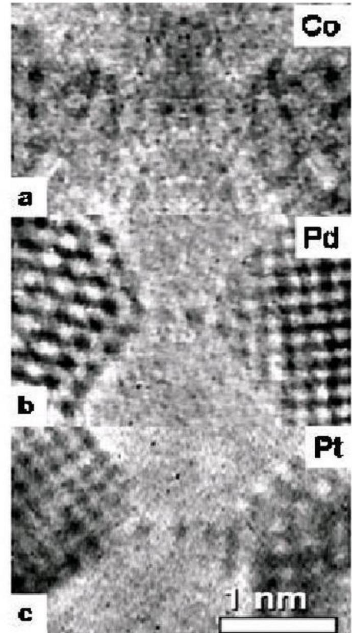
FIG. 2. HRTEM atomic resolved images showing the formation of suspended chains of atoms just before the contact rupture. (a) Co. (b) Pd. (c) Pt.
