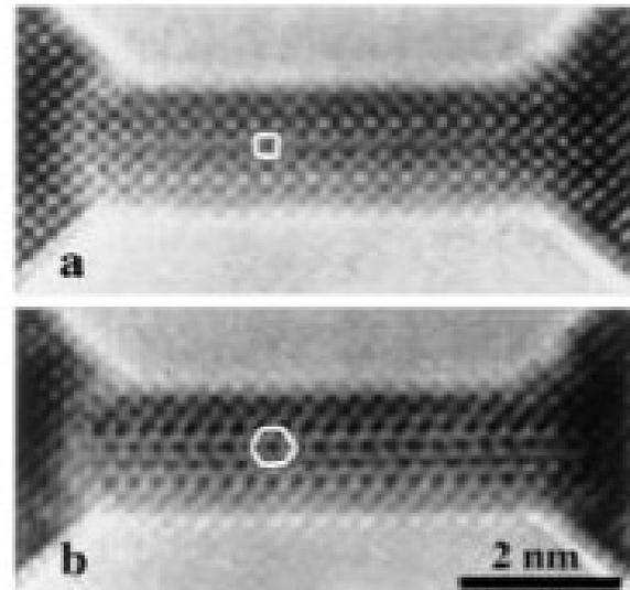
FIG. 2. Transmission electron micrographs of an Nb 2 nm thick; obtained at the focuses of (a) 65 nm and (b) 55 nm. Note the square lattice in (a) and hexagonal one in (b).
