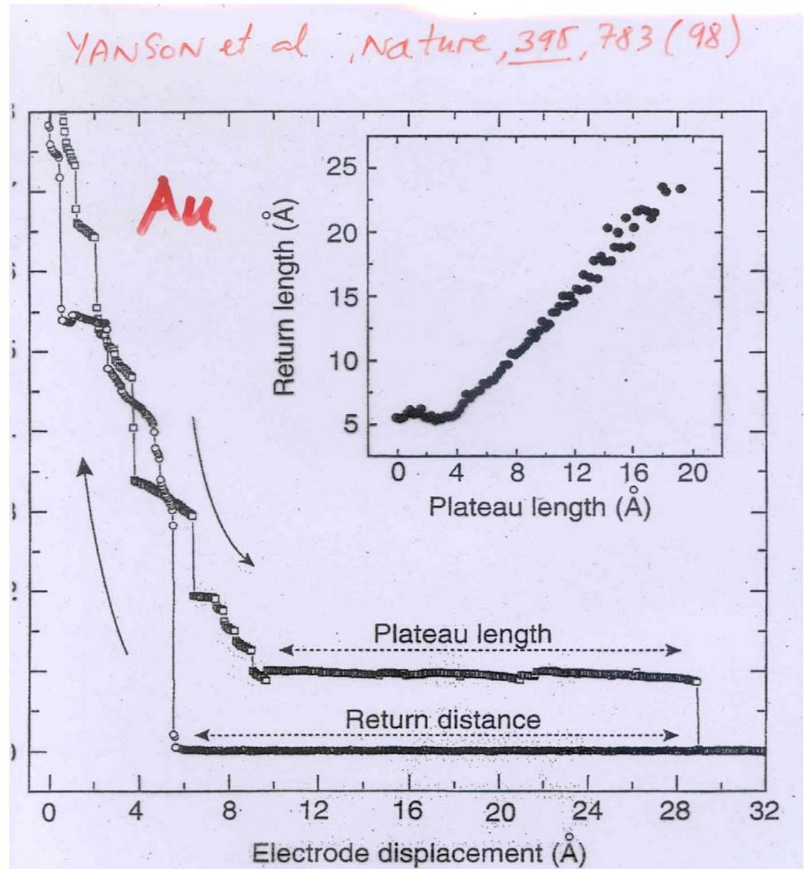
1 Conductance as a function of the displacement of the two gold electrodes with respect to each other in an MCB experiment at 4.2 K. The trace
