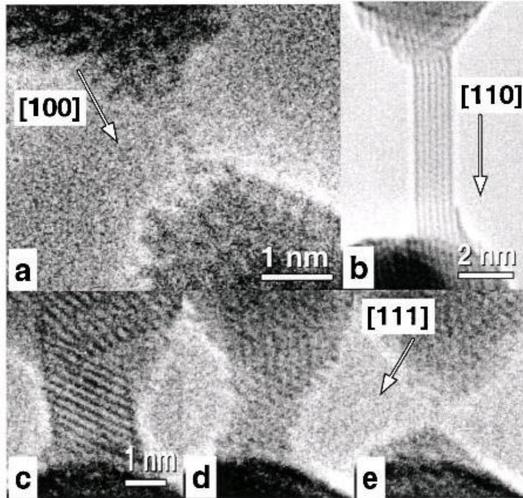
FIG. 2. HRTEM images of gold NWs; atomic positions appear dark. (a) [100] atom-chain NW; (b) rodlike [110] NW; (c)–(e) temporal evolution of a NW formed when the apexes are sliding: 0, 17:12, and 24:15 min, respectively.
