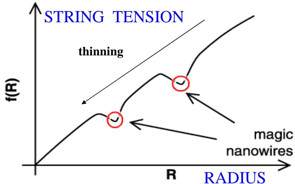
**Fig. 1.** String tension of a tip-suspended nanowire as a function of radius (schematic). Local minima signal long-lived magic nanowires. The wire disappears ( $R = 0$ ) at true equilibrium.
