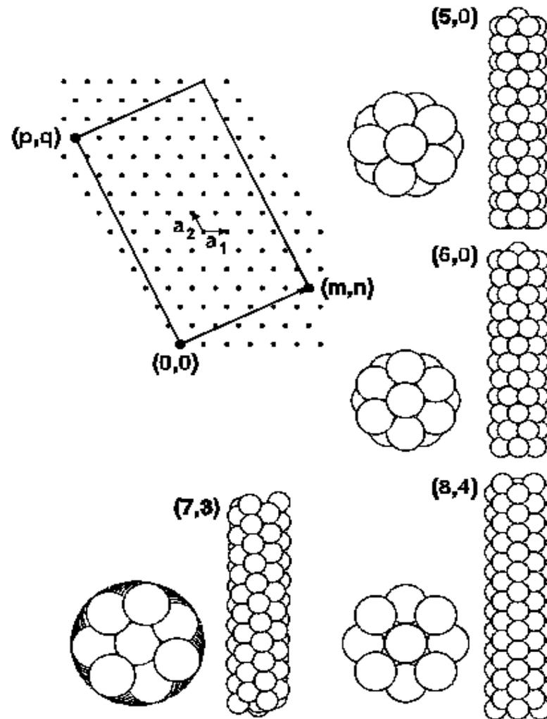
**Fig. 2.** Cylindrical folding of a triangular lattice for an  $(m, n)$  tube, with views of several coaxial tube nanowires. Each atom is pictured as a sphere of atomic radius. The  $(7, 3)$  gold nanowire (note its chirality) was reported to be magic in (3).
