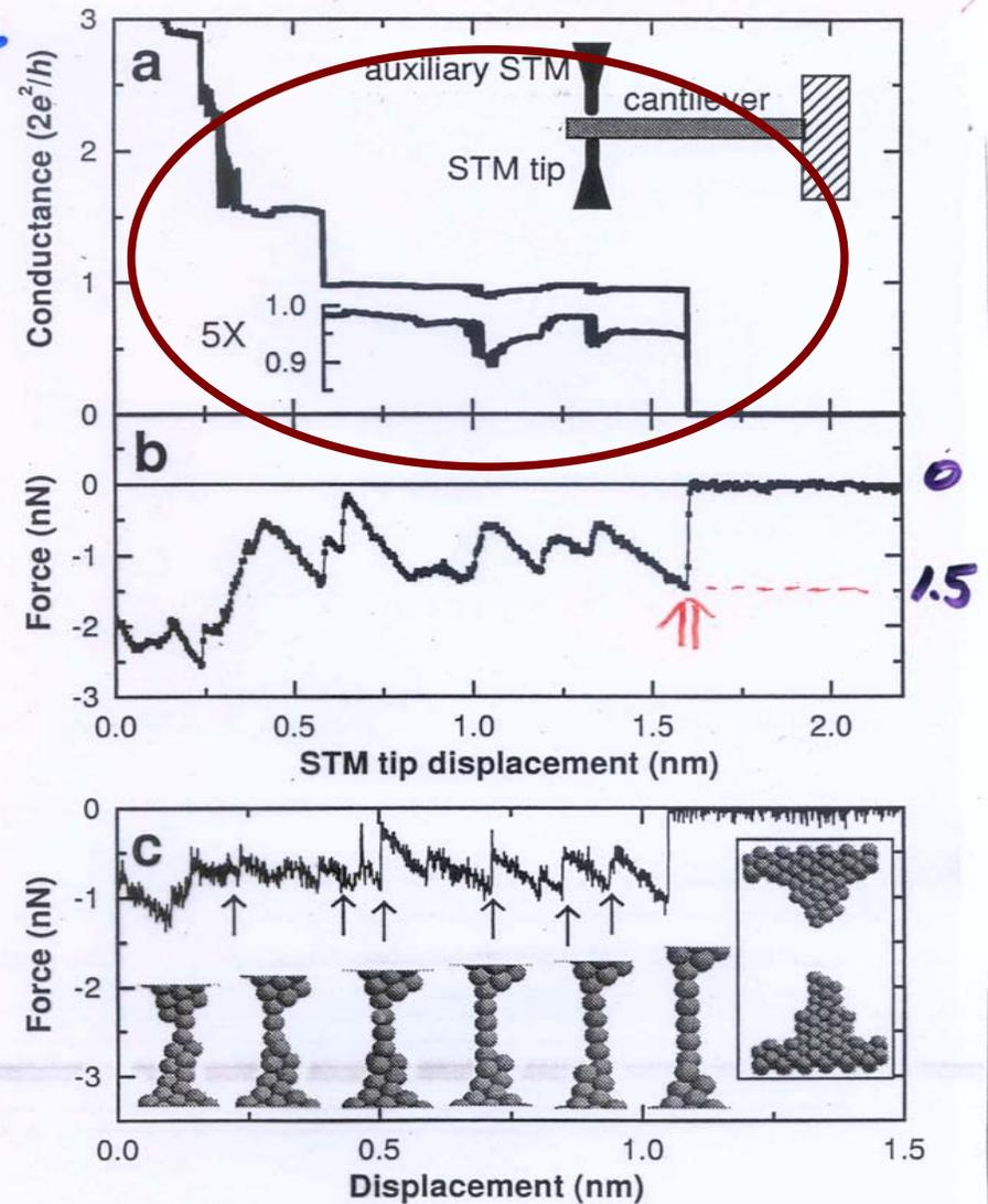
FIG. 1. Simultaneous conductance (a) and force (b) measurement during chain fabrication and breaking. The conductance in the last plateau has been zoomed to show detailed variations. Inset: schematic drawing of the experimental setup. (c) Calculated force during the MD simulation.
