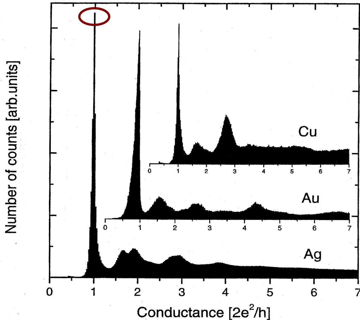
**Figure 3.6:** Conductance histograms for pure copper, silver and gold constructed from >1000 individual conductance traces each. The measurements were performed at 4.2 K and 100 mV bias voltage. Total amplitudes of the histograms are scaled to fit; relative amplitudes of the peaks within each histogram
